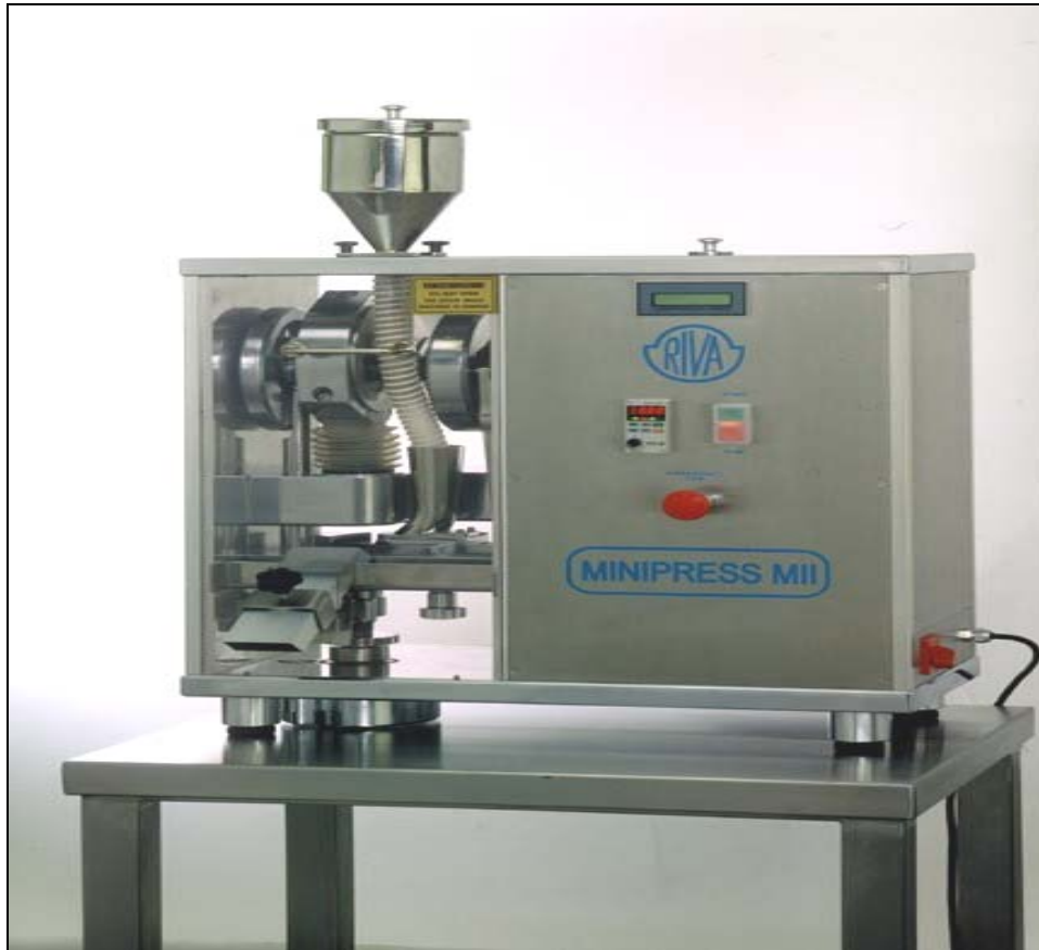
Riva-Minipress , single punch excenter press
